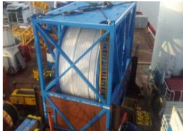
Spoolable pipeline products (Airborne Oil & Gas)
