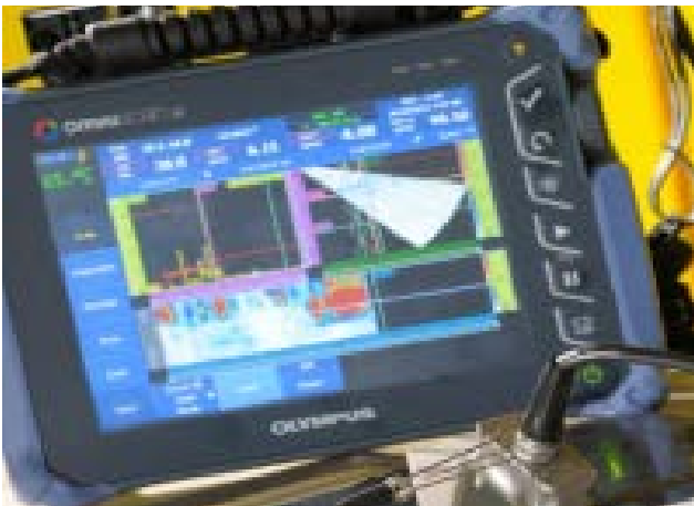
Phased-array ultrasonic testing (TWI Ltd)
