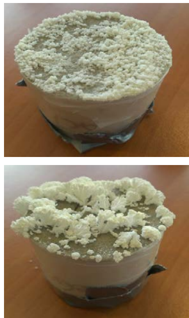
Figure 7: Effects of novel crystal growth inhibitors on halite deposition in porous media and control without inhibitor (bottom). Images courtesy of TNO.
