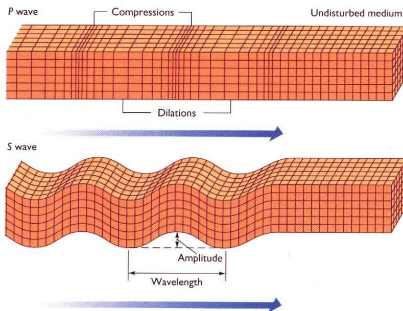
Figure 5. Propagation modes of P-waves and S-waves
