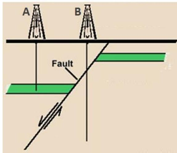
Figure 2. Schematic diagram of two wells in a fault zone; in the event of an earthquake on this fault, well B will clearly suffer damage.
