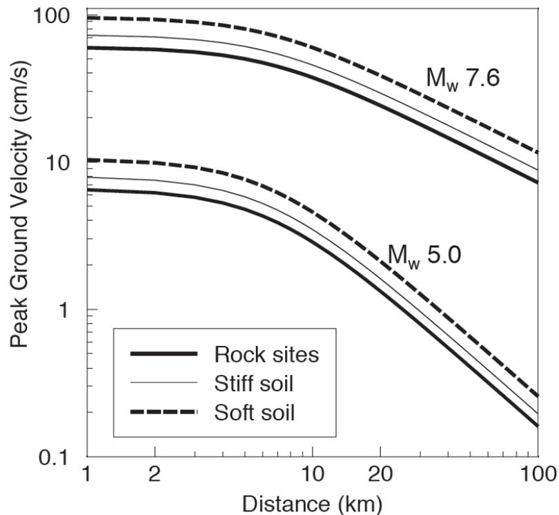
Figure 7. Predicted PGV values (in cm/s) as a function of magnitude, distance and site classification (Akkar & Bommer, 2010)
