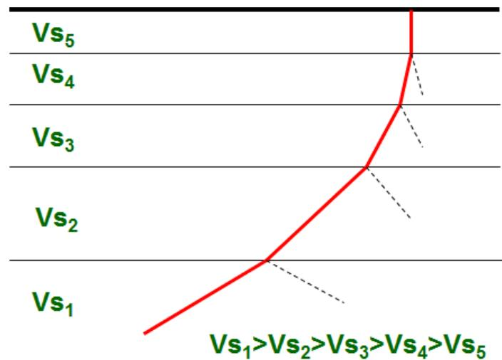
Figure 6. Propagation of an S-wave upwards through layers of decreasing velocity near the ground surface; the wave path, indicated by the red lines, is refracted into a near-vertical direction. The dashed lines indicate the wave energy reflected from the interface between the layers
