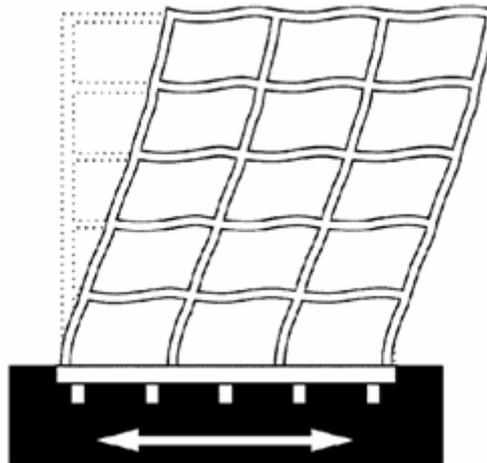
Figure 1. Schematic illustration of how horizontal ground motions leads to vibration in a building and displacement of the structure relative to its foundations, resulting in deformation of the structural elements
