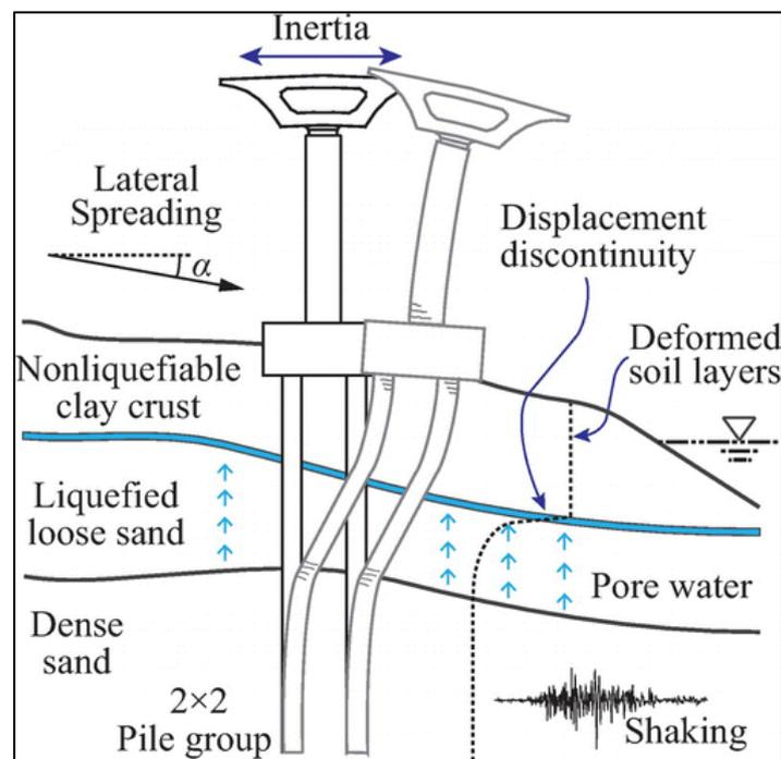
Figure 4. Schematic illustration of piles below a bridge pier being deformed by lateral spreading of a liquefied sand layer
