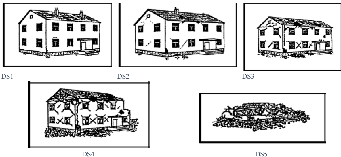
Figure 2.9. EMS damage grades for URM buildings (Grunthal, 1998). DS1: non structural damage, such as hairline cracks in plaster; DS2: initiation of structural damage, with cracks in many walls; DS3: moderate structural damage wherein most walls have large and extensive cracks; DS4: very heavy structural damage is present, with serious failure of walls, and partial structural failure of roofs and floors; DS5: near total collapse.
