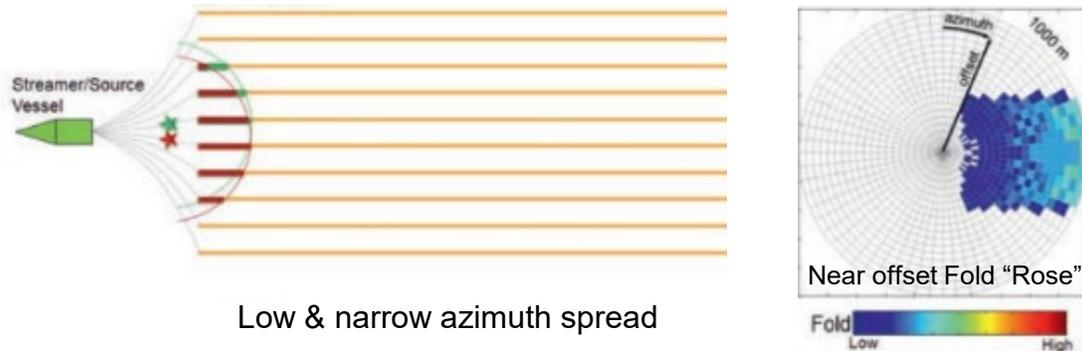
Low & narrow azimuth spread
