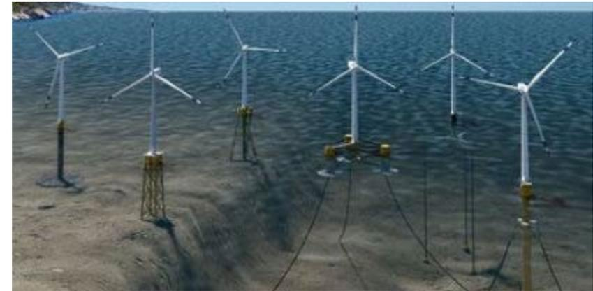
3D image showing range of wind turbines and foundations. Catenary cables & multiple anchor points, tension leg turbines OBN equipment fragile/ NOAR not laid over catenaries. AUV, ROV needed.
