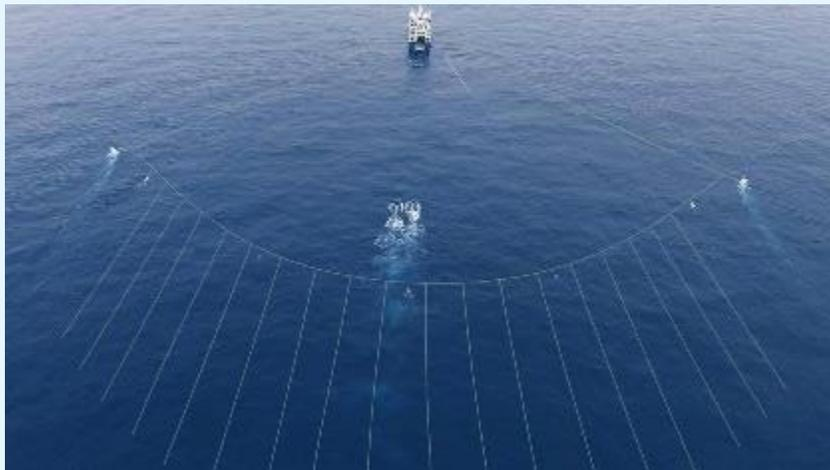
18x100m cables with tow width of ~200m
