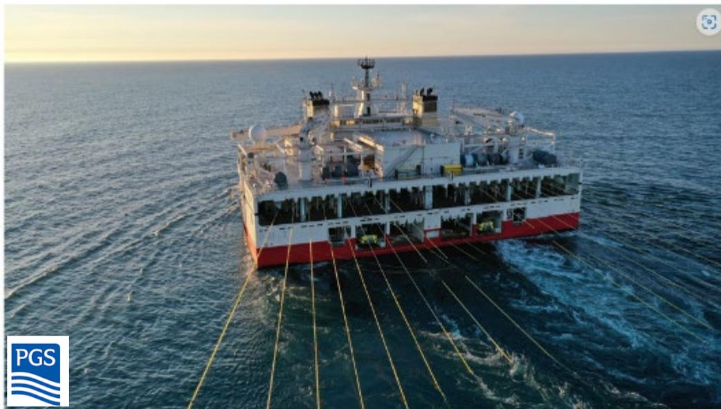
Ramform Hyperion towing 18 x 75m x 8 025m GeoStreamer spread.
